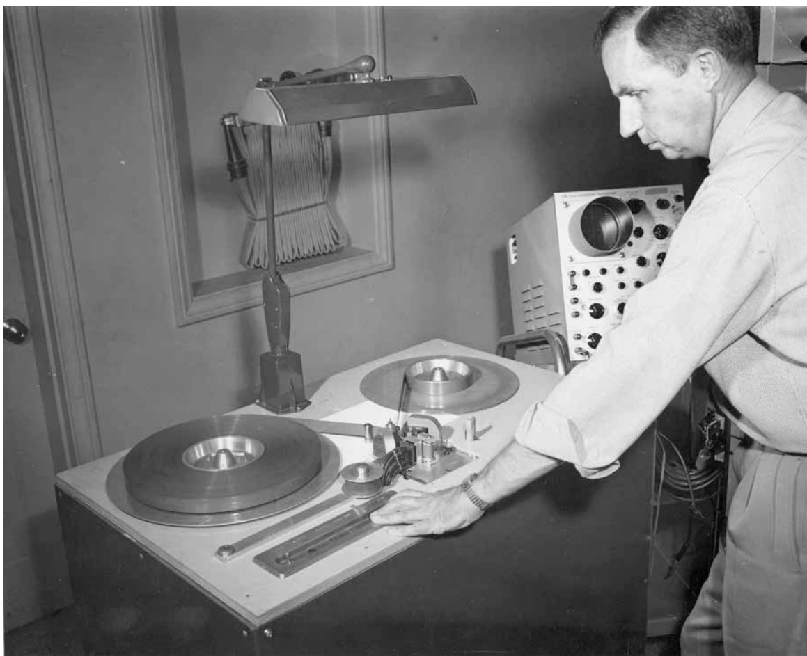
Jack Mullin and an early version of the Crosby video recorder that operated at 360 inches per second recording twelve tracks on a tape one inch wide.
